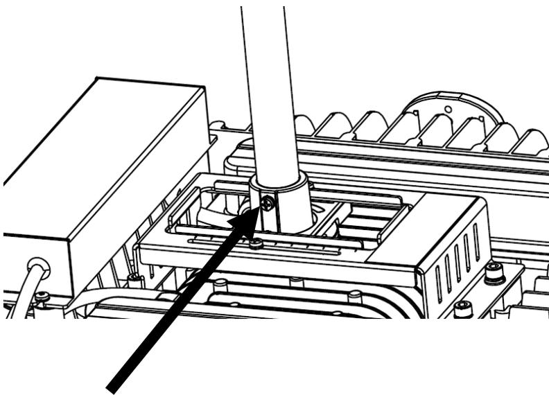
3. The fixture should already be factory set for correct balance and orientation. If adjusting balance or orientation is necessary, make corrections using the adjustment screws in the locations shown
