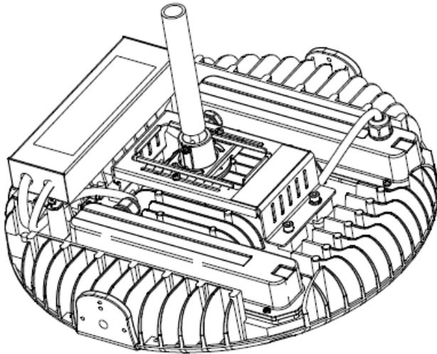
2. Insert set screw in order to secure the fixture to the Pipe.
